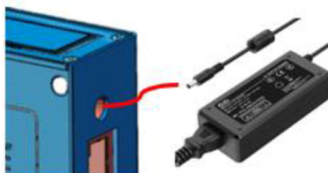
Figure Connecting the power supply through the independent power supply interface.
